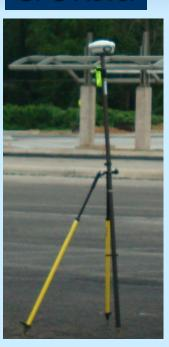
Real Time Kinematic (RTK) GPS Precision
