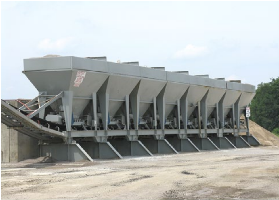
FIGURE 5.6 TYPICAL COLD FEED SYSTEM
