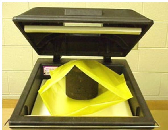
FIGURE 4.23 VACUUM SEALING DEVICE
