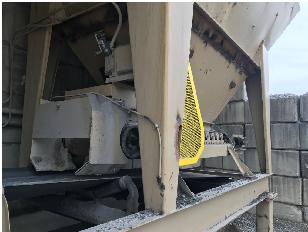
FIGURE 5.7 CONTINUOUS BELT FEEDER
